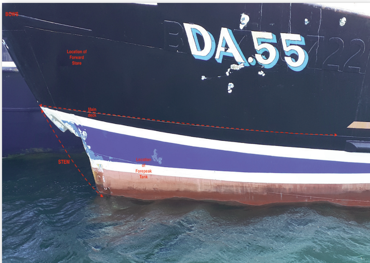
Photograph No.2 - Bow damage above the waterline.
