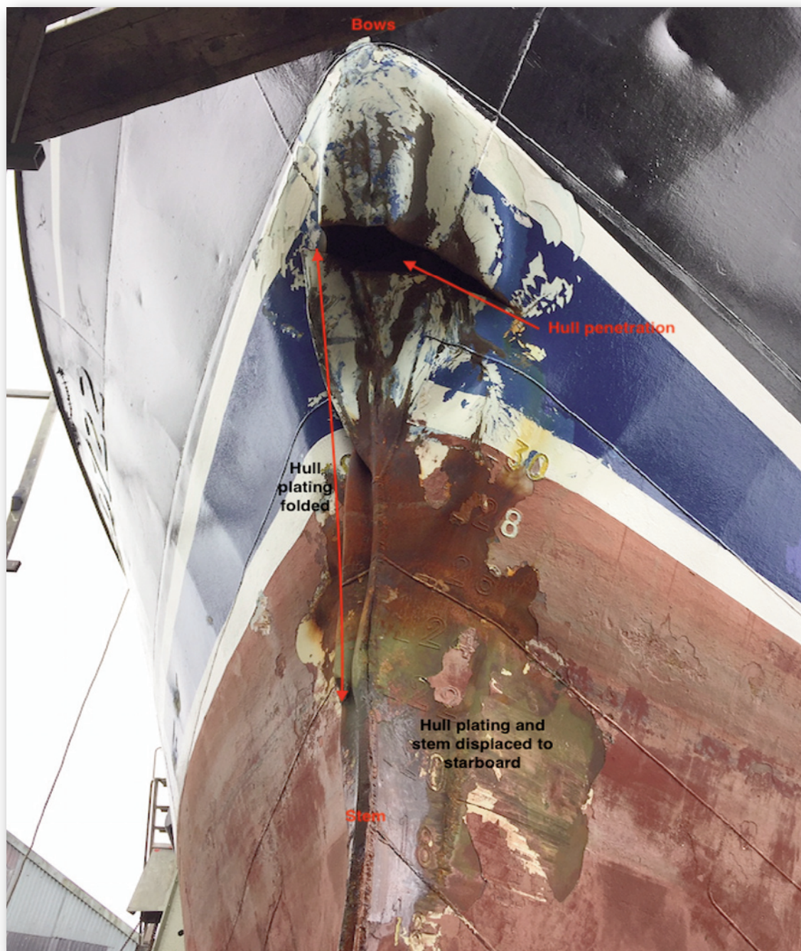
Photograph No.4 - Stem damage below the waterline.
